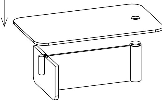
When moving the table, do not lift the table top, lift from the base.
